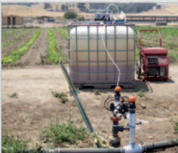
The Chem-Pro diaphragm metering pump's small size provided a simple solution in this high pressure, high output fertigation application.
